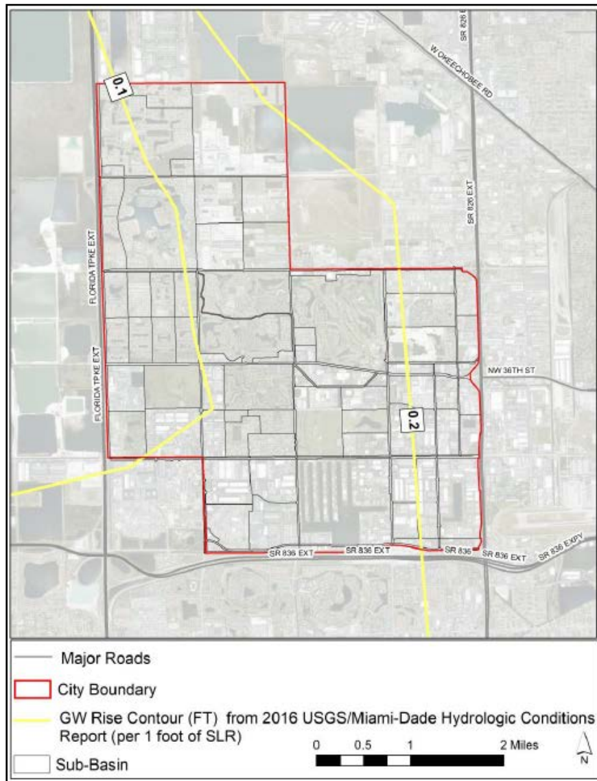
Figure 6-3 – October Average Groundwater Rise Contours with One Foot of Sea Level Rise
